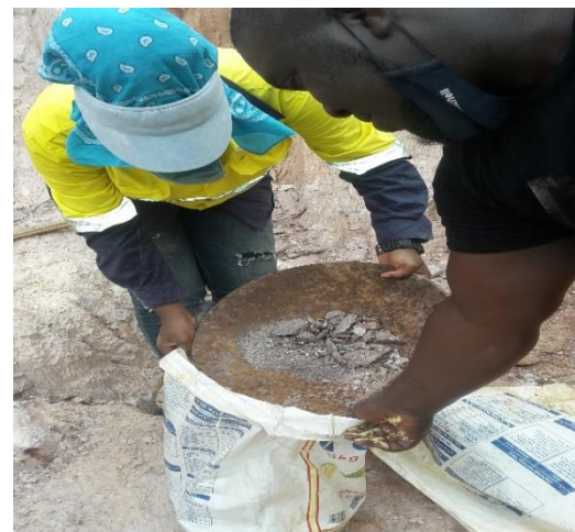
Photo 4 breaking down large rocks into small chips photo 5 quartz rocks collected in a rice bag
