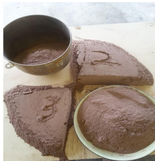
Figure 3 coning and quartering ( Abhishek Kumar,n.d.) photo 14 laboratory scale coning
